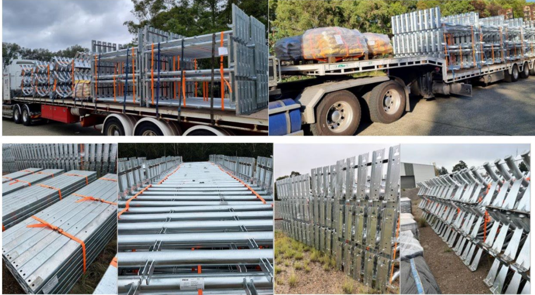
Delivery of belt structure for underground conveyors
