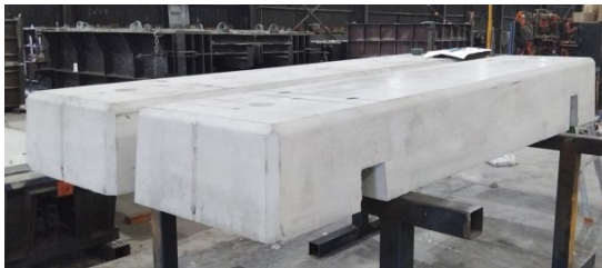
Manufacture of components of overland conveyor structure
