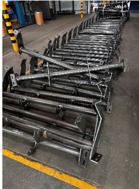
Manufacture of components of overland conveyor structure
