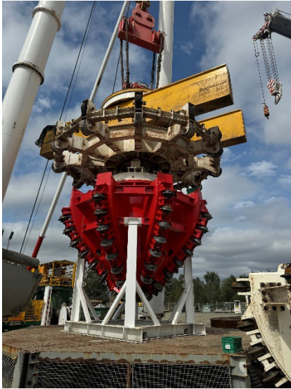
Drill rig for LW ventilation shaft
