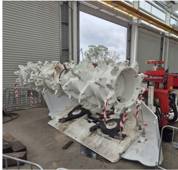
Continuous Miner final assembly & commissioning
