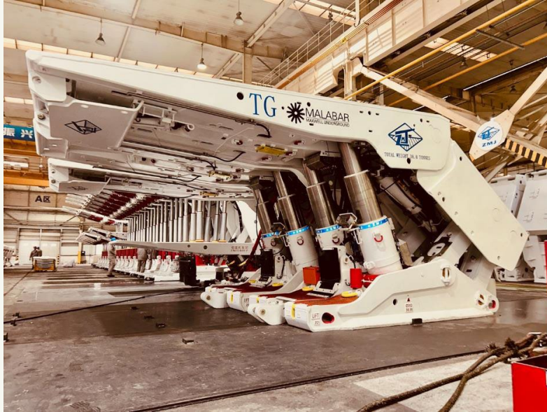
Longwall roof support inspection in China
