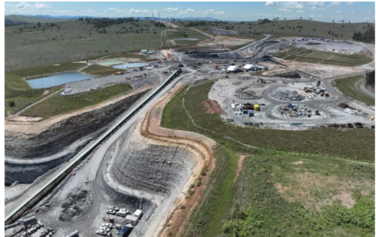
Underground mine entry area (MEA). Note progressive establishment of vegetation and pastures within the MEA
