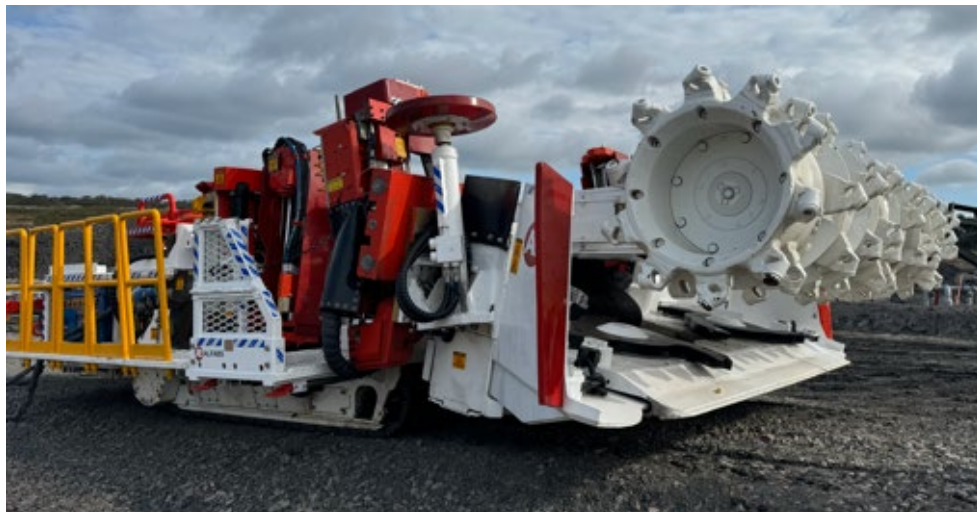
Continuous miner for developing the longwall roadways at site
