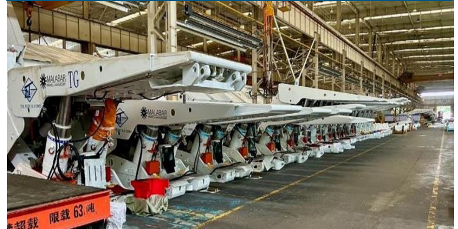
Longwall roof supports in China
