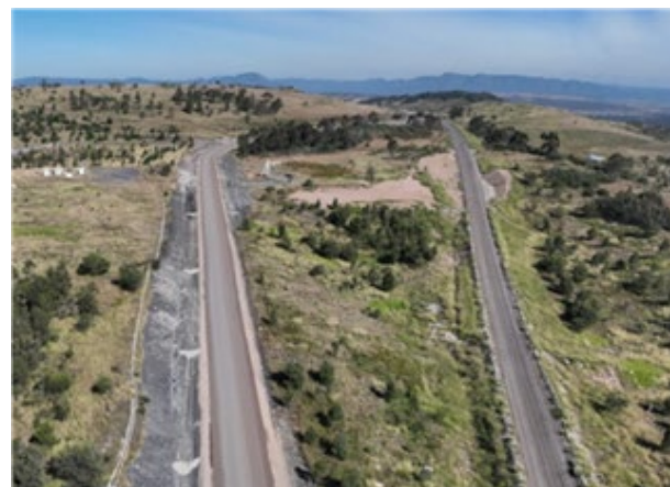
Sealed permanent access road (shown on left) overland conveyor trace (shown on right)
