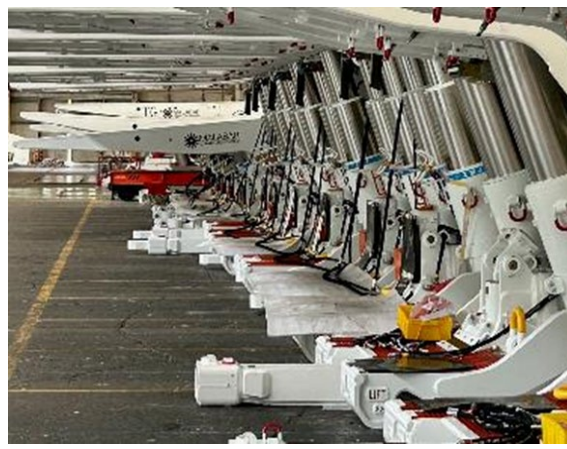
Longwall roof supports following completion of line build in China; expected to land in Australia September 2024
