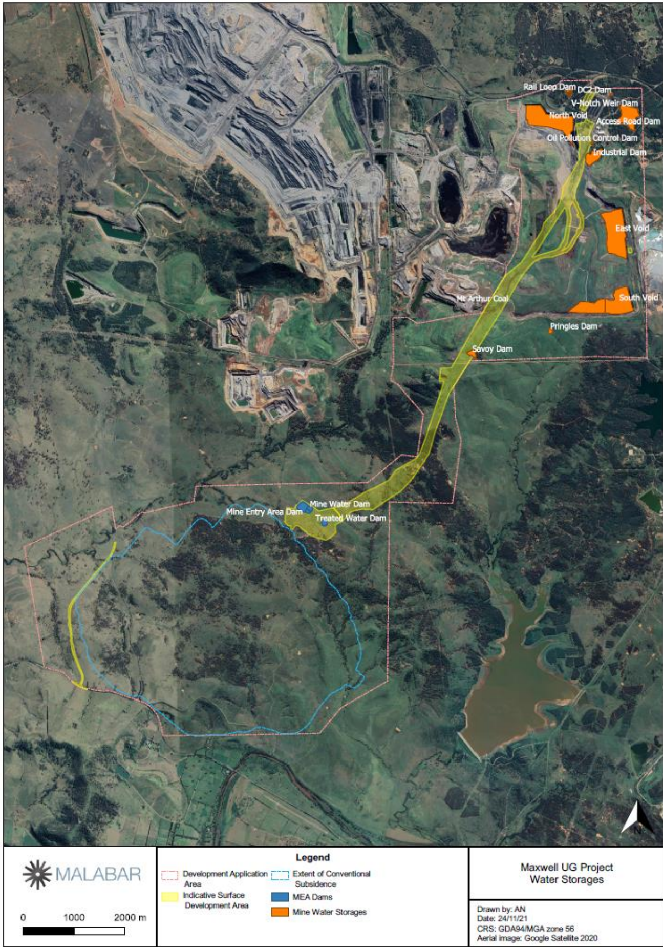
Figure 2: Existing and proposed mine water storages
