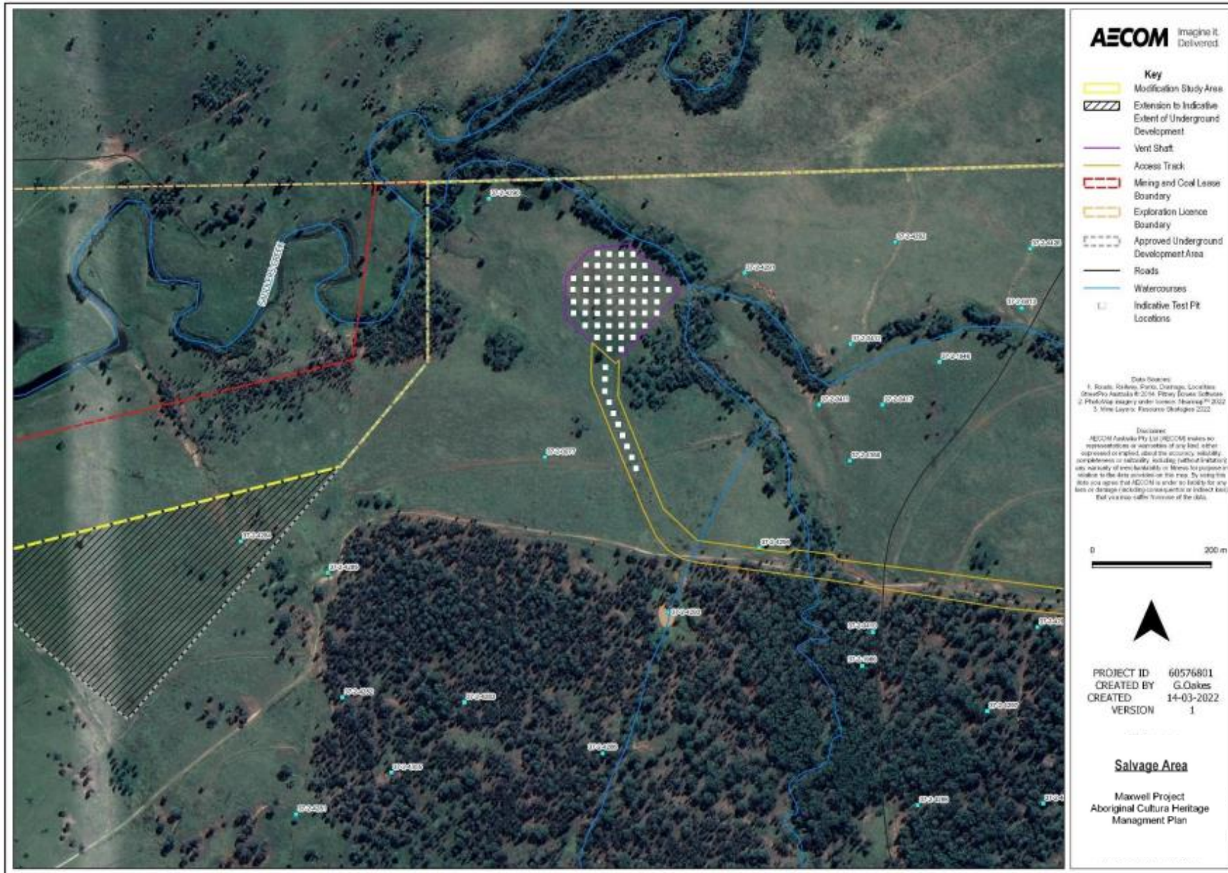
Figure 6. Indicative test pit locations for the upcast ventilation shaft and access
