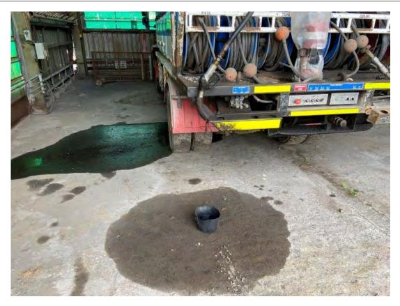
Plate 27 - Fuel and oil leaking from fuel cart during site inspection
