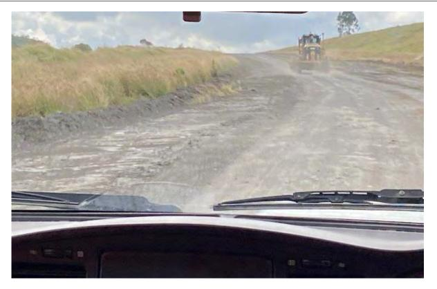
Plate 39 – Wheel generated dust from mobile plant on haul road
