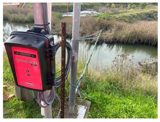
Plate 2 - Rail loop dam level indicator
