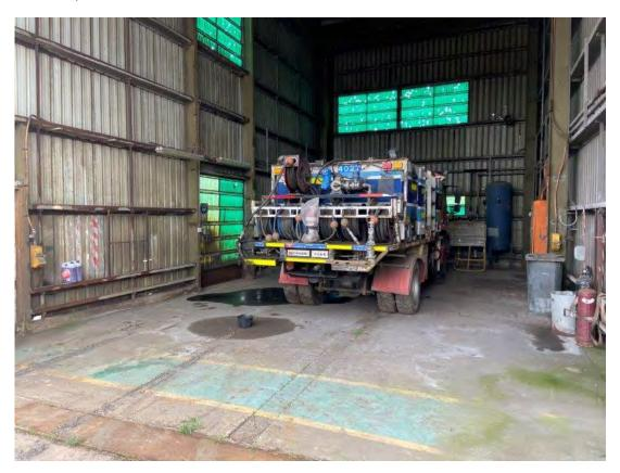
Plate 26 – Fuel and oil leaking from fuel cart during site inspection
