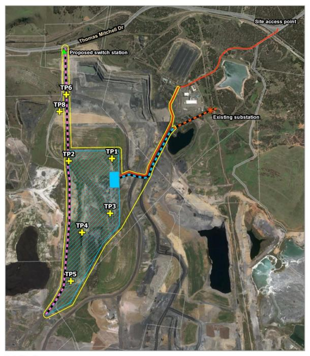
Test pit locations 19-069 Maxwell Solar Farm Test pit Project boundary Indicative solar array Indicative battery storage Proposed 66kV line Proposed 33kV line Existing 33kV line
