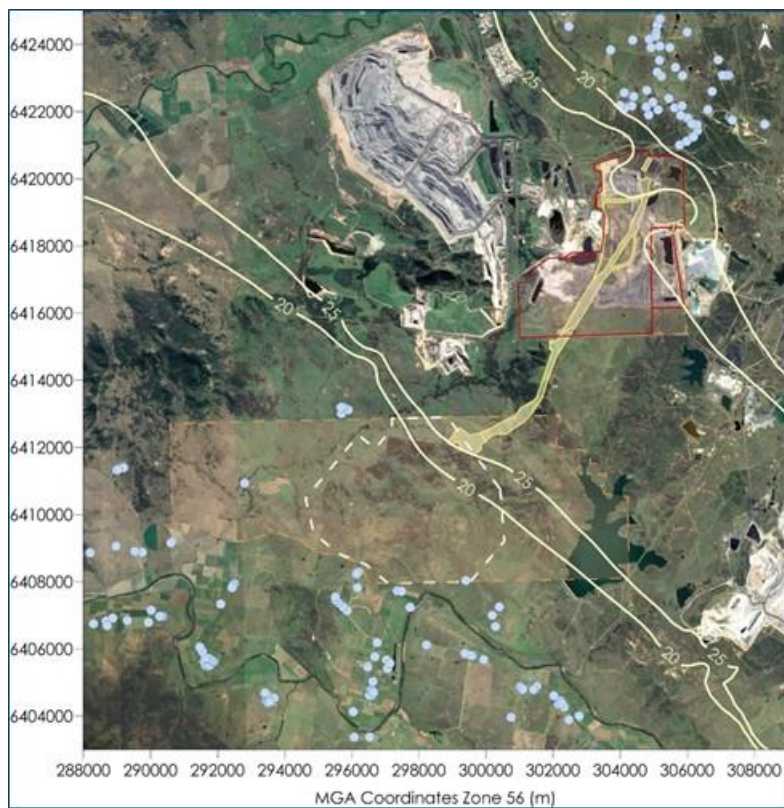
Figure E-26: Predicted annual average PM 10 concentrations due to emissions from the Project and other sources in Scenario 3 ( \mu\text{g}/\text{m}^3 )
