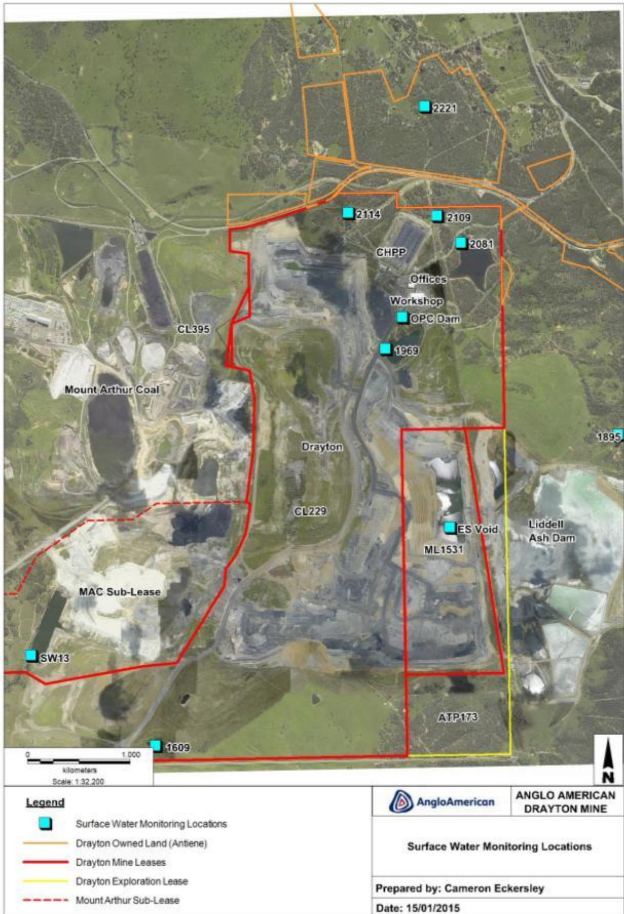
Figure 12: Surface water monitoring sites
