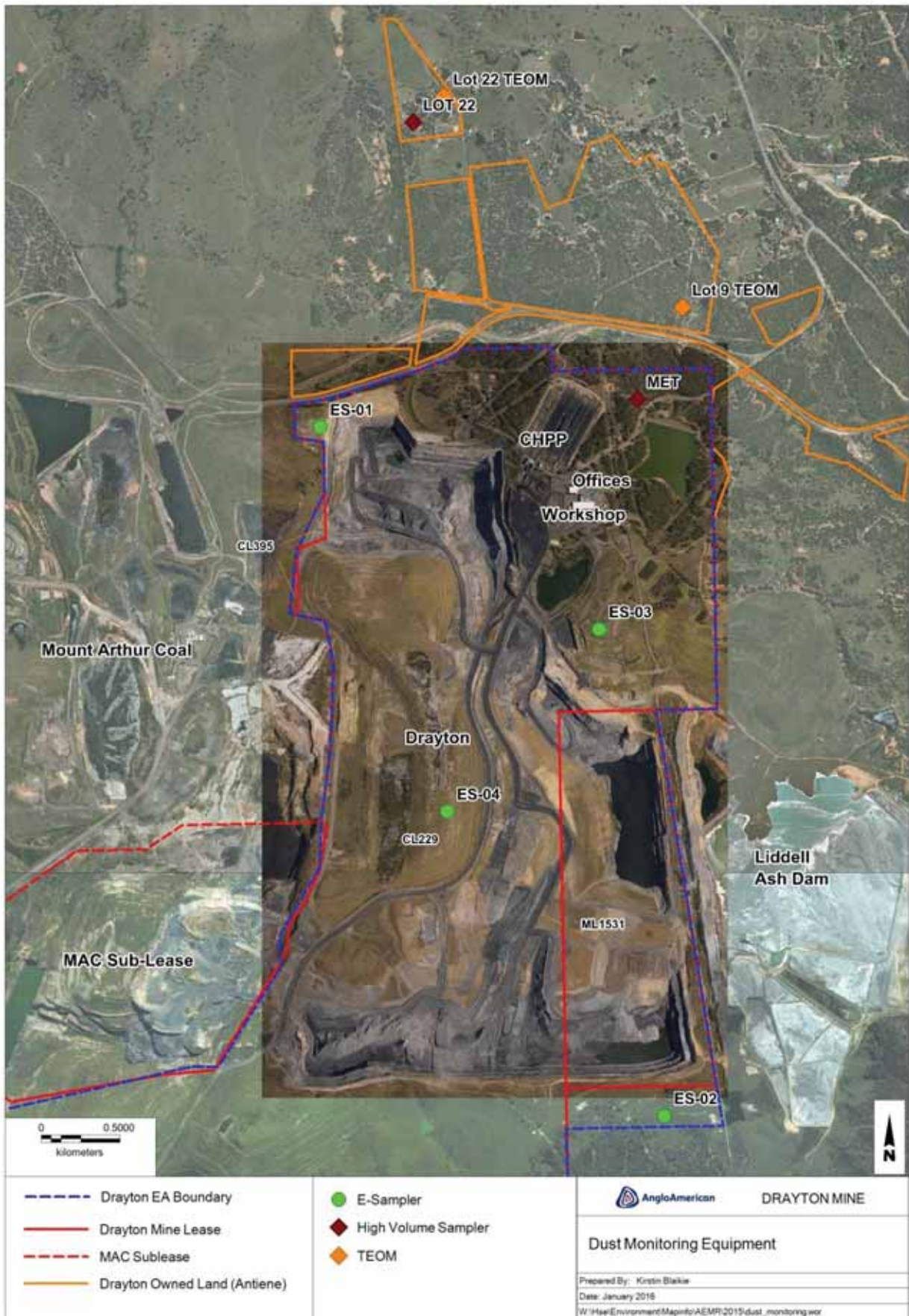
Figure 7: Real-time Dust Monitoring Equipment
