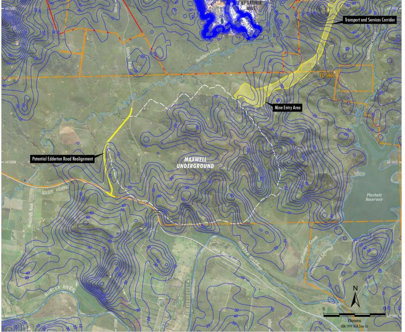
LEGEND Exploration Licence Boundary Mining and Coal Lease Boundary Indicative Surface Development Area Extent of Conventional Subsidence (20 mm subsidence contour) Depth to Water (m)
