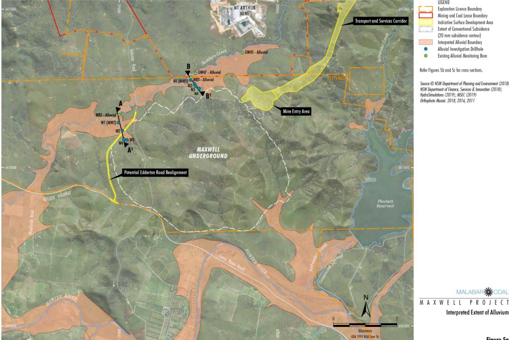
IFGEND Exploration Licence Boundary Mining and Coal Lease Boundary Indicative Surface Development Area Extent of Conventional Subsidence (20 mm subsidence contour) Interpreted Alluvial Boundary Alluvial Investigation Drillhole Existing Alluvial Monitoring Bore
