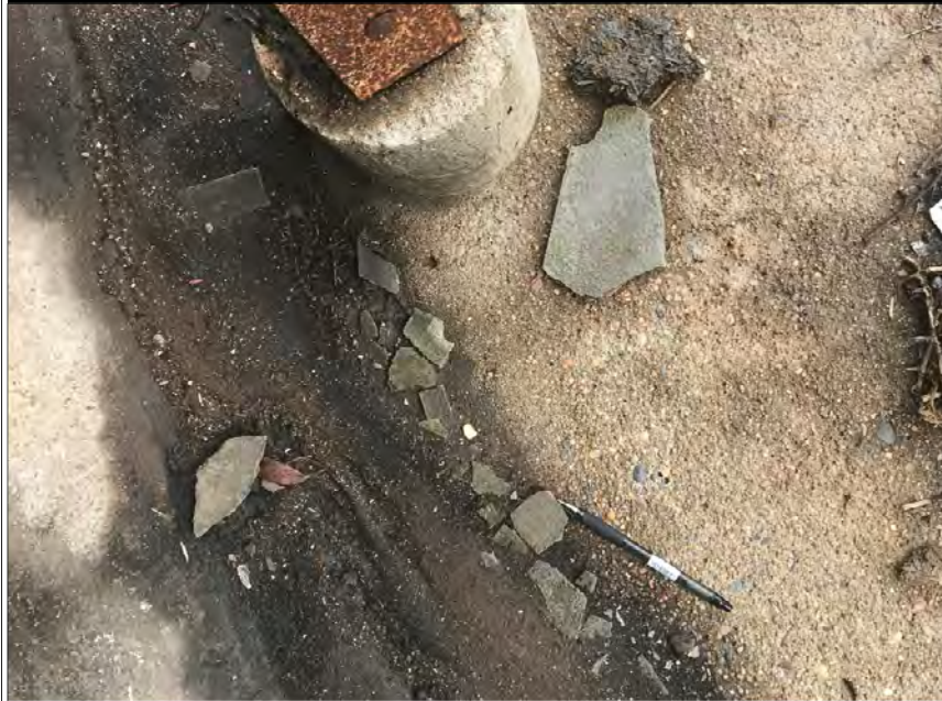
PHOTOGRAPH T: POTENTIAL ACM ON FLOOR OF STEEL SHED
