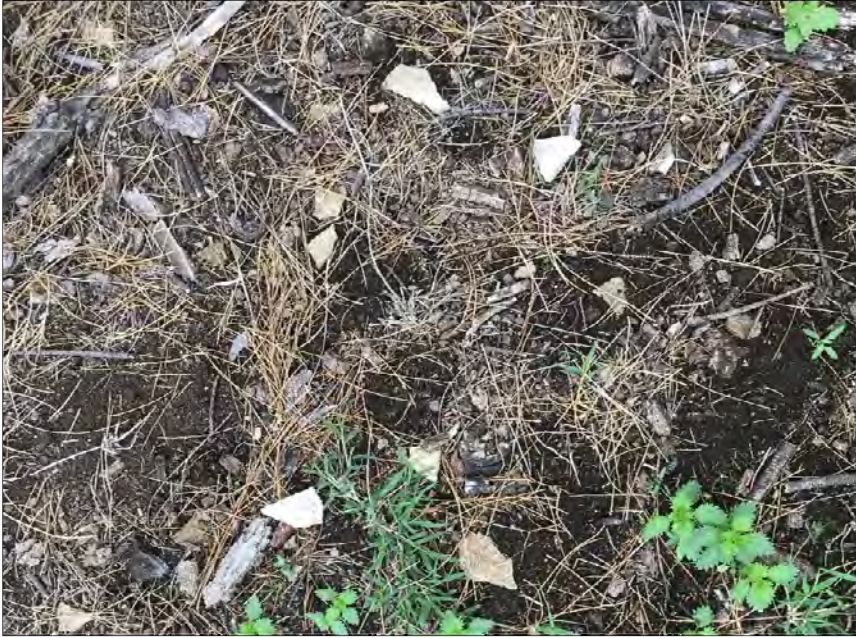
PHOTOGRAPH M: ACM FRAGMENTS ADJACENT TO NISSEN HUT
