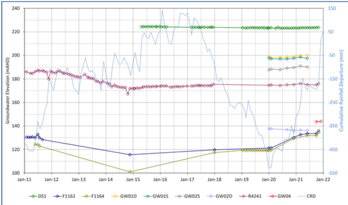
Figure 15. Long-term groundwater levels – Maxwell Infrastructure
